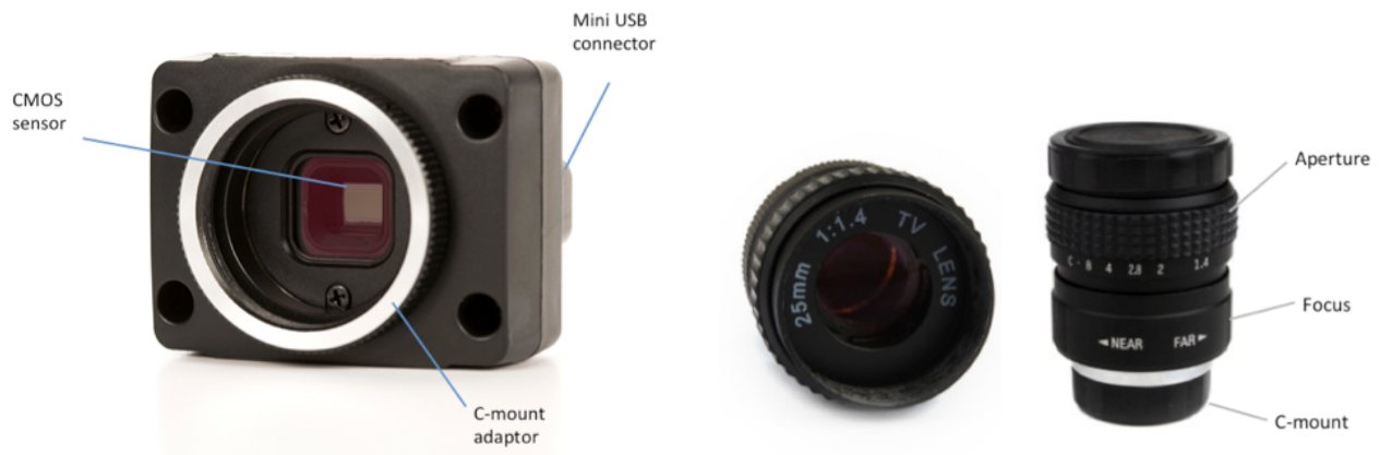
Fig. 3.— (left) The Point Grey Flea sensor. The light gray area at the center is the CMOS detector array. (right) The 25 mm camera lens. The lens has a C-mount which screws into the image body. This component has a built-in aperture stop, which can be adjusted by a ring on the body. The C designation means closed. There is also an adjustable focus barrel.
