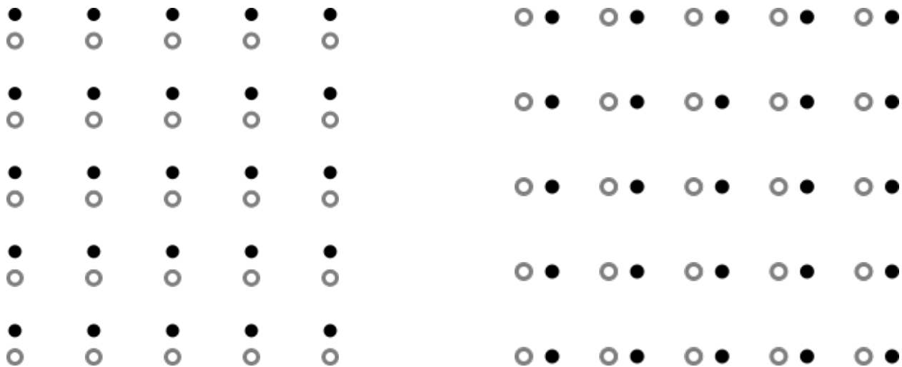
Fig. 7.— Displacement of spots for tip and tilt modes. The spot displacements are all the same, since the phase gradients across each subaperture are equivalent.
